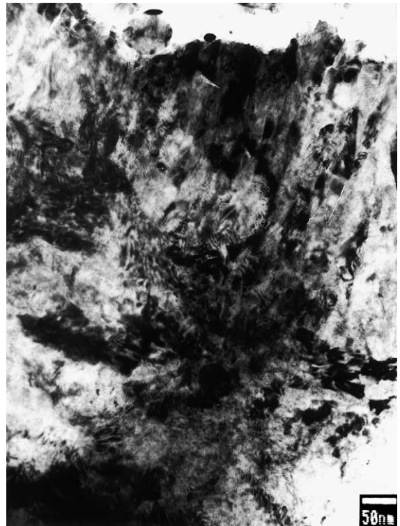
Fig. 8. TEM micrograph of sample Zry-2:D after oxidation at 360°C for 96 h.
