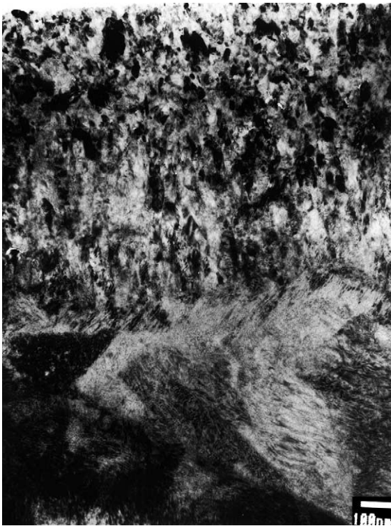
Fig. 7. TEM micrograph of sample Zry-2:C after oxidation at 360°C for 96 h.
